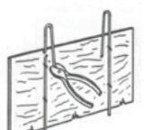
1. Remove broken fastener by cutting wire.
