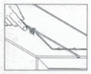
Cut the twist remaining on the ends of the binding wires. Insert the end of the wire on top of the box into the coiled ends of the Roebuck Splioer.
