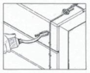
Using a twisting tool such as the Bruce Twister shown here, twist the wires tightly together. The excess wire ends are clipped off automatically. A few turns will be sufficient.
