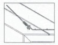
Draw the end of the binding wire through as shown in the illustration and then bend it into a hook form with the end of the wire pointing back in the Roebuck Splicer coils.
