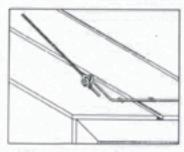
Pull the Roebuck Splicer away from the hook, making sure that the end of the hook fits into the other half of the coil. When this is drawn tight the splicing is securely completed.
