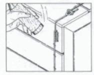
The result will be a good tight twist with smooth ends. Using a hammer or the handle of the twister, knock the twists down safely against the side of the box.
