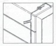
Bringing the spliced wire ends over the box corner, draw the opposite ends together about one-half inch below the top of the box. The wires are then bent as illustrated to engage the tool.
